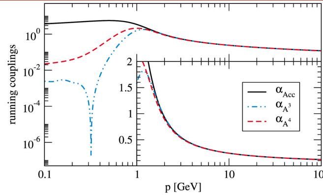
(b) Effective running couplings, [721], as obtained from different Yang-Mills vertices: three-gluon vertex:  $\alpha_{A3}$ , four-gluon vertex:  $\alpha_{At}$ , ghost-gluon vertex:  $\alpha_{A\bar{c}c}$ . At large momenta the couplings agree due to universality.
