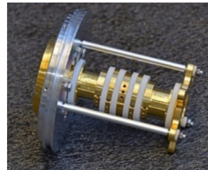
Second trap (accumulation/selection/measurement)
