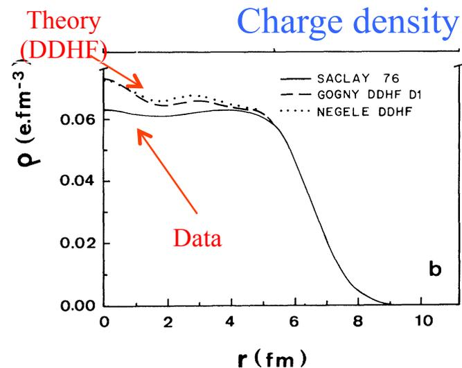
Very precise determination of the charge density down to  $r = 0$  fm
