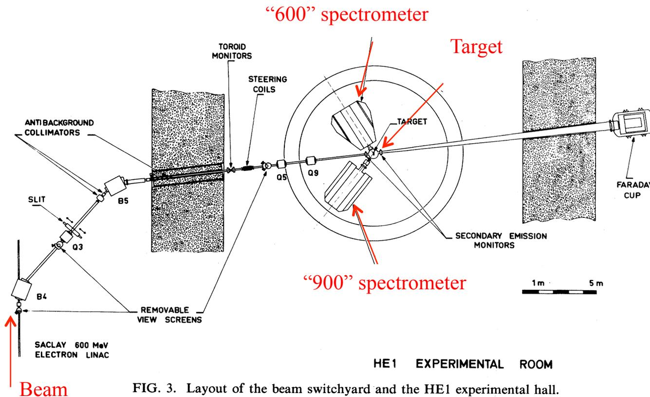
FIG. 3. Layout of the beam switchyard and the HE1 experimental hall.
