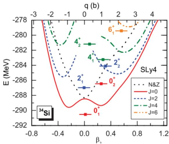
FIG. 1. (Color online) Energy curves for the particle-number-projected HFB states (N&Z) and particle-number and angular-momentum projected states ( $J = 0, 2, 4, 6$  curves) for  $^{34}\text{Si}$  as a function of the intrinsic quadrupole deformation of the mean-field states they are projected from. The solid square dots correspond to the lowest GCM solutions, which are plotted at their average deformation  $\sum_q q |g_\mu'(q)|^2$  (see text).
