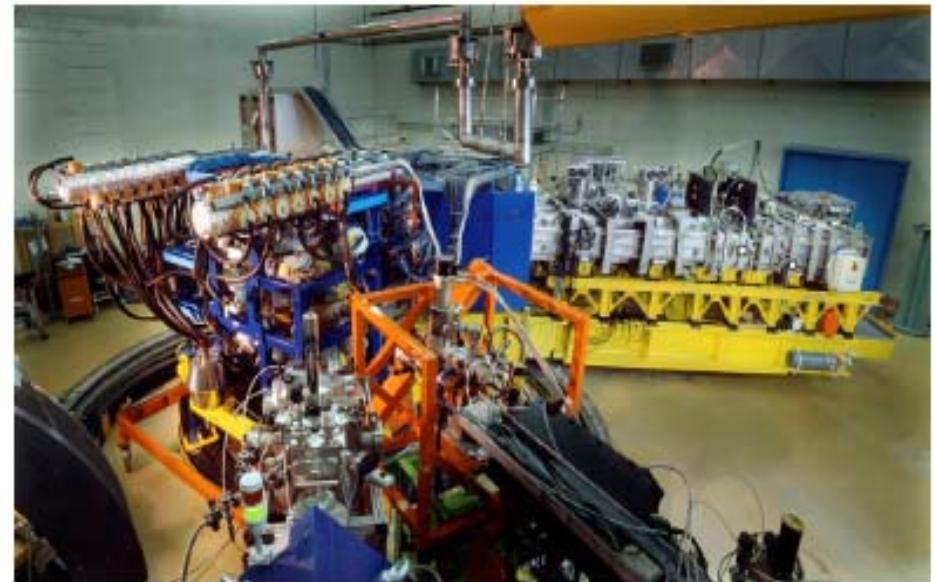
Figure 1. View of the CLARA-PRISMA setup. The CLARA array of Clover detectors is on the left, followed by the quadrupole and dipole magnets, and the focal plane detector of PRISMA can be seen on the right.
